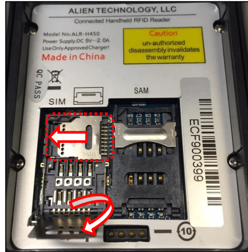
FLIP the SIM card holder up toward you out of the way. SLIDE the SD card holder toward the left to release it.
