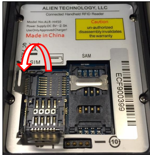
FLIP the SD card holder up toward the left.
