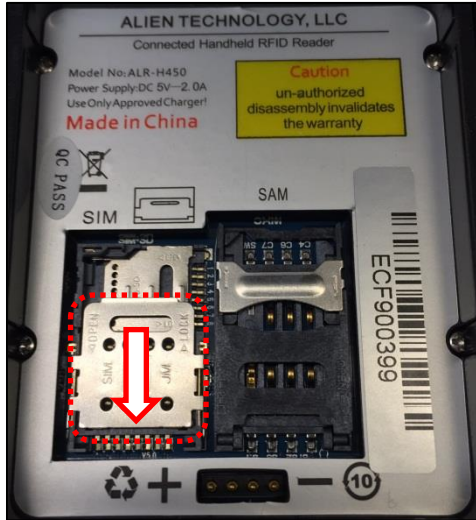
Locate the SIM card holder and SLIDE it downward to release it.
